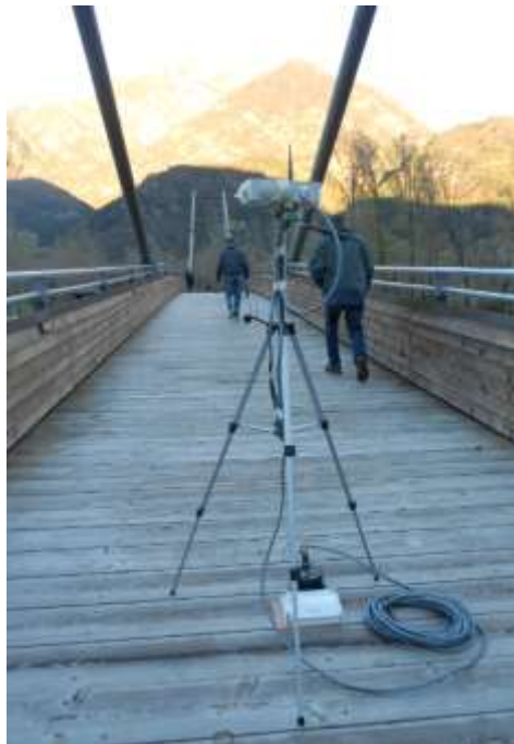
Figure 3.1.13. The tri-axial accelerometer connected with a wireless sensor unit (WSU) posed over the deck.
