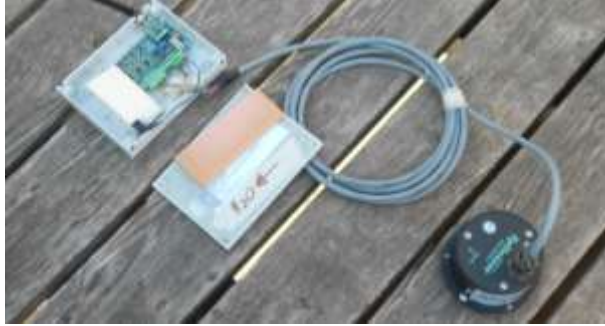
Figure 3.1.2. Example of the wireless station unit (WSU) employed for the data acquisition-transmission.
