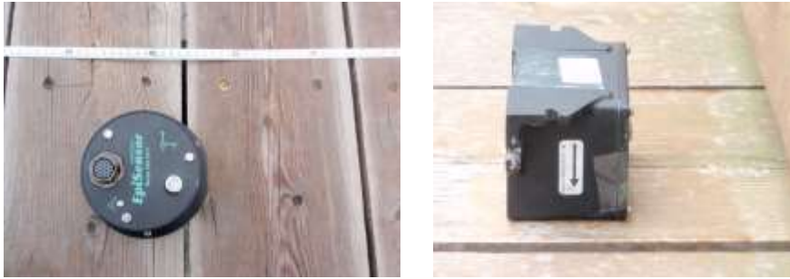
Figure 3.1.14. Example of the Kinematic EPISENSOR uni- and tri- axial accelerometer employed during the experimental campaigns.
