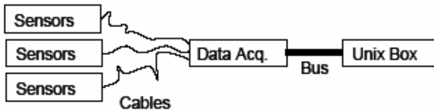
Figure 4.1 Today's conventional wired monitoring system.
