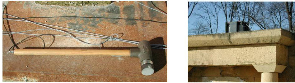
Figure 9.7 Forced excitation methods. (a) Instrumented hammer. (b) Shaker at the top of the structure, in central position.
