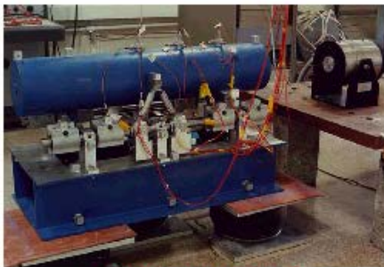
(c) An electro-dynamic shaker:
