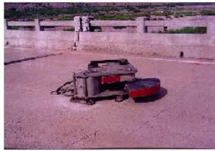
(b) Mechanical eccentric mass shaker: generates sinusoidal excitation, but difficult to apply in vertical direction.
