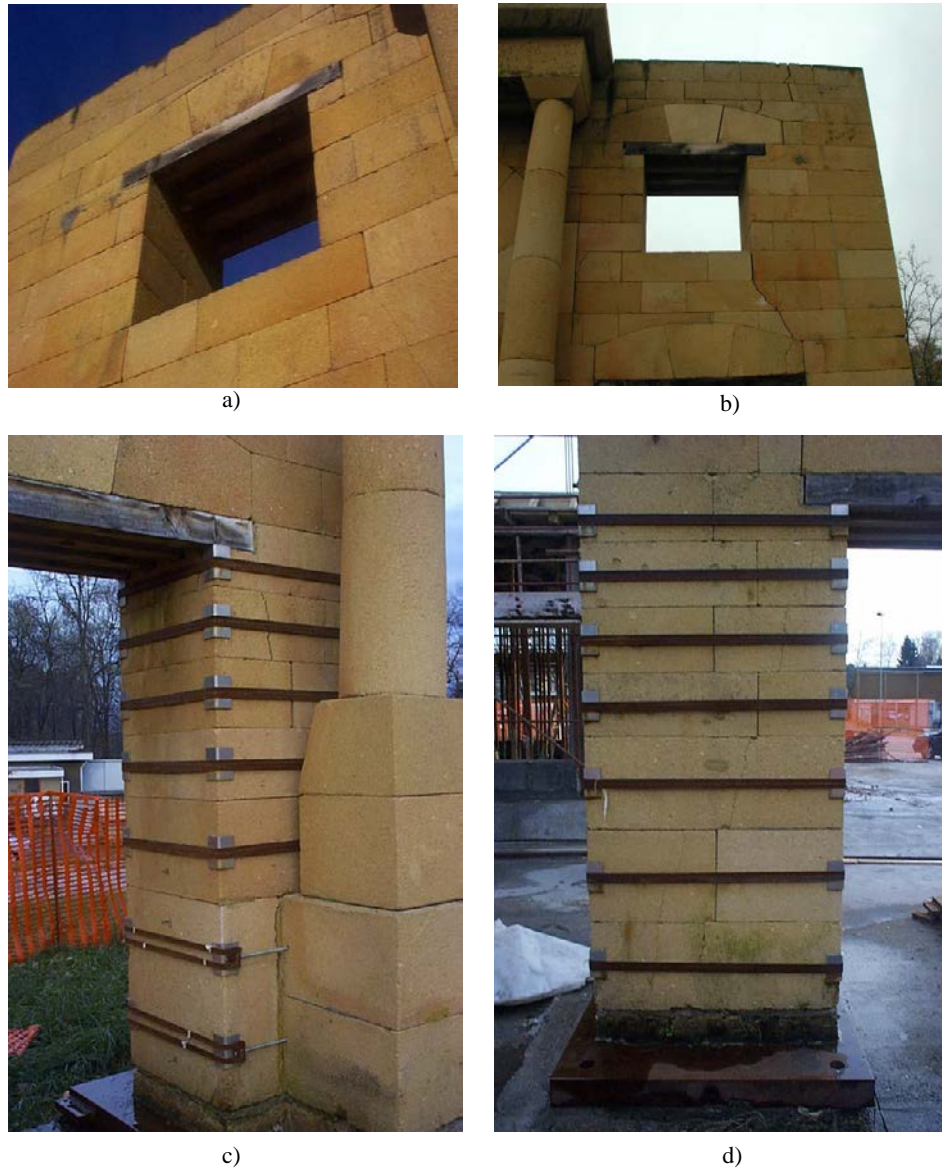
Figure 9.4 Cracks at different locations of the reduced model: (a) left openings; (b) right openings; (c) central-left foot; (d) right-end foot (through cracks on the rear side).
