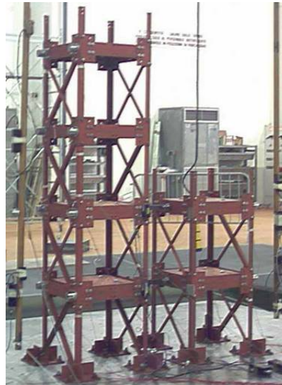
Figure 9.1 Structural models (scale 1:5) of steel buildings
