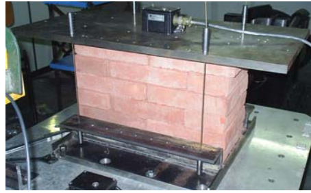
Figure 3.16: Tested wall with two SMA wires at the corners.
