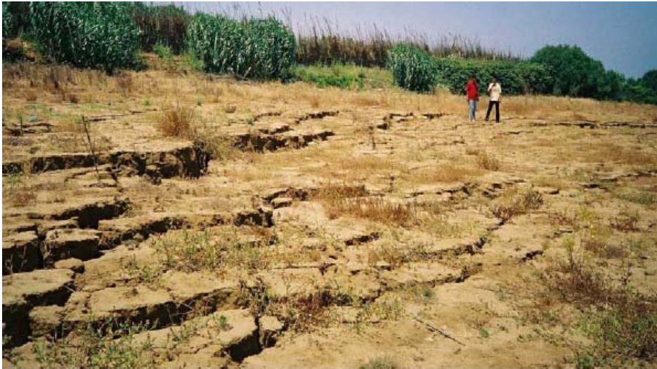
Figure 2.12: Lateral spreading in the epicentral area of the May 21, 2003 earthquake close to the Zemmouri-El-Bahri port.
