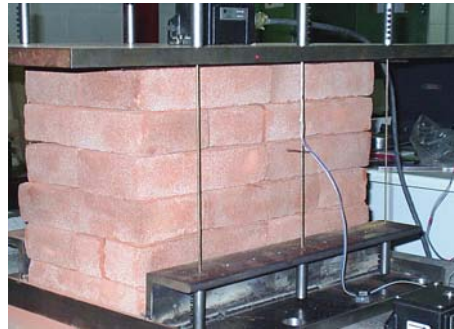
Figure 3.17: Tested wall with three equidistant SMA wires.
