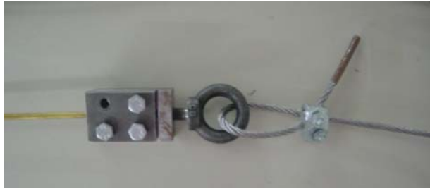
Figure 4.15: Connection of the steel cable to the SMA wire.
