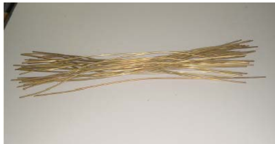
Figure 4.14: Sixty centimetres long SMA wires of diameter 3.5 mm.
