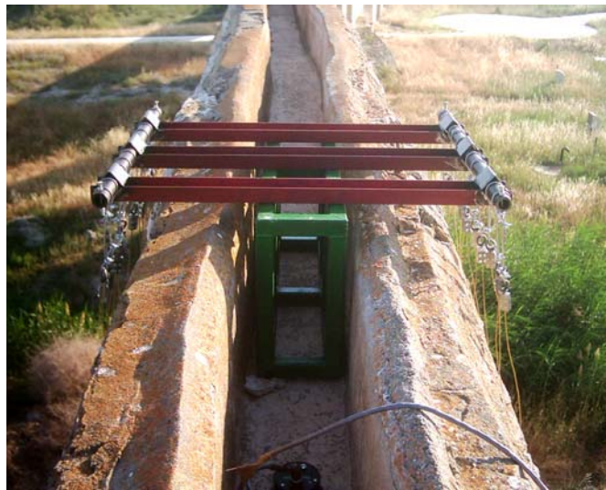
Figure 4.13: Rigid base to support the upper end of the SMA pre-stressing assembly.
