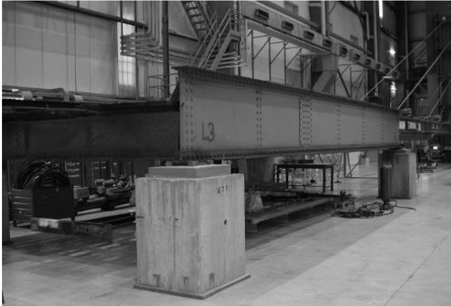
Figure 5.31: The Rohrbach bridge (CaSCo3 mock-up) installed inside the ELSA laboratory
