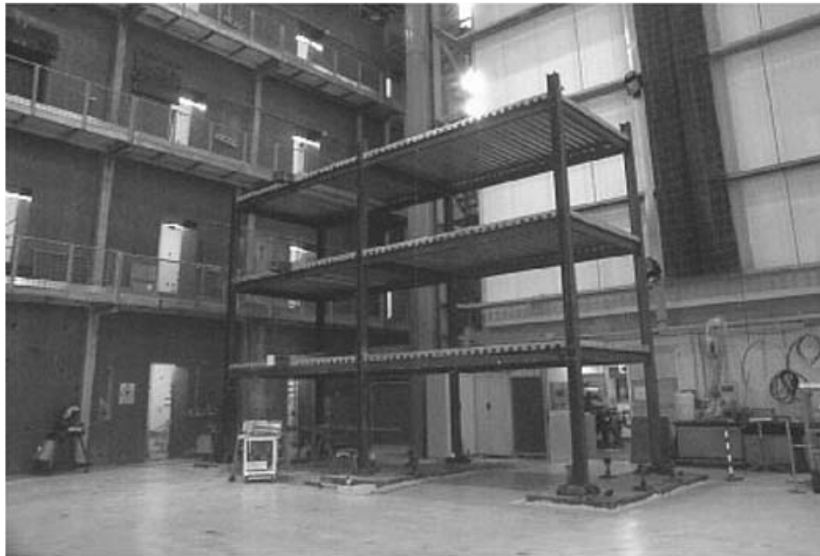
Figure 5.19: The Baby-Frame structure in front of the Reaction Wall at ELSA (without energy dissipators)
