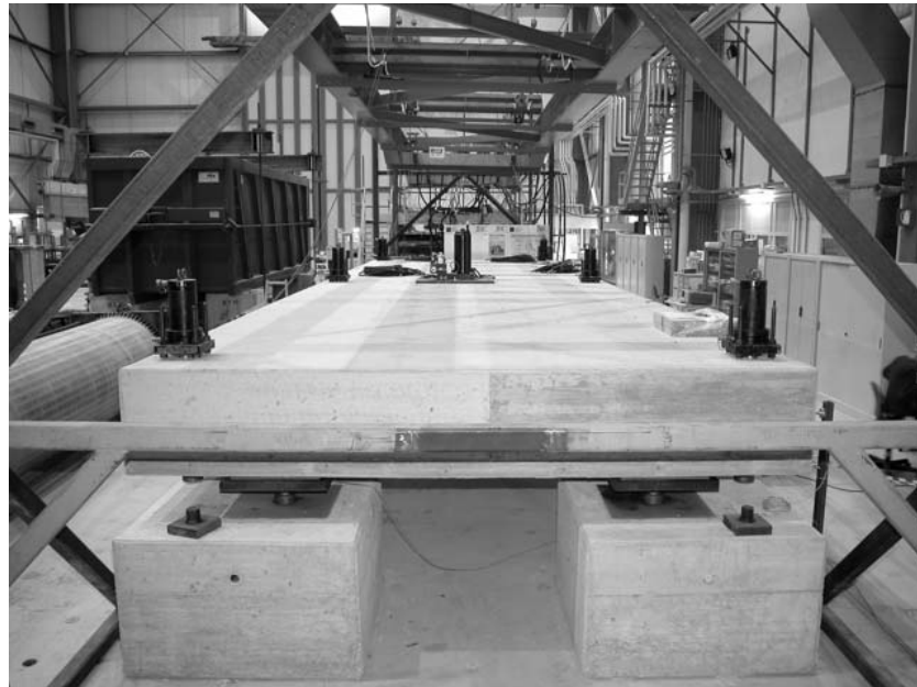
Figure 5.30: The Mass-Spring System (CaSCo2 mock-up)
