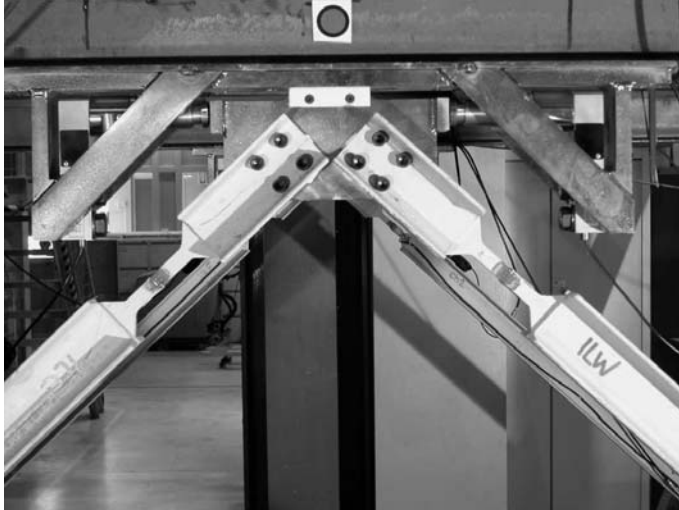
Figure 5.22: Passive JARRET device installed on the Baby-Frame
