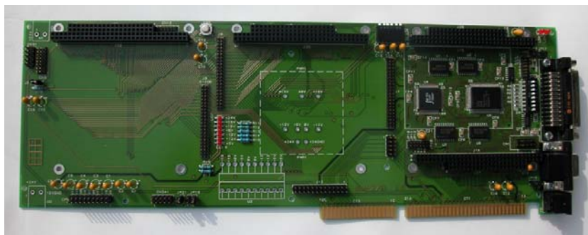
Figure 4.6: Slave card without modules (the Dual-RAM is visible on the left side)
