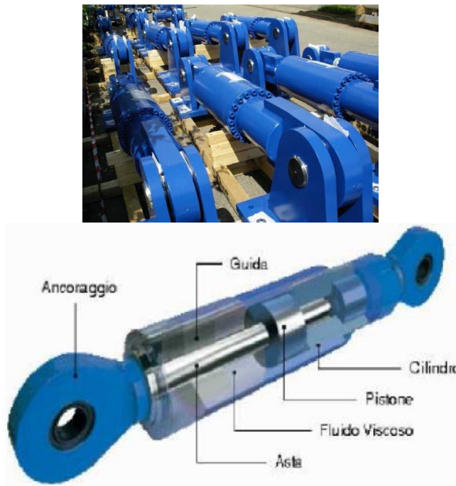
Figura 1-42: Viscous fluid damper
