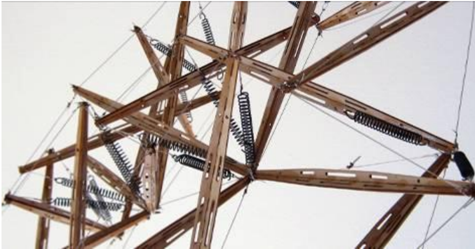
Figure 2.12 – Actuated tensegrity prototype by Tristan d'Estree Sterk and ORAMBRA, 2009.
