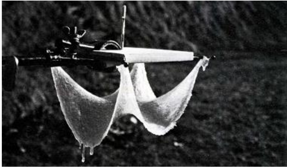
Figure 3.1 – Hanging model by Heinz Isler.
