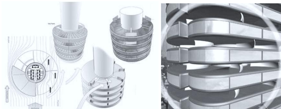
Figure 5.4 – Vertical axis wind turbines between each floor for energy harvesting; the building aims to be sustainable and self-powered other than aesthetically pleasant (Fischer, 2008).
