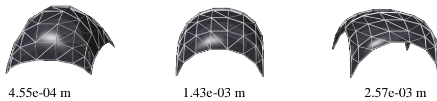
Figure 6.9 – Three reference configurations and the respective maximum values of deflections.
