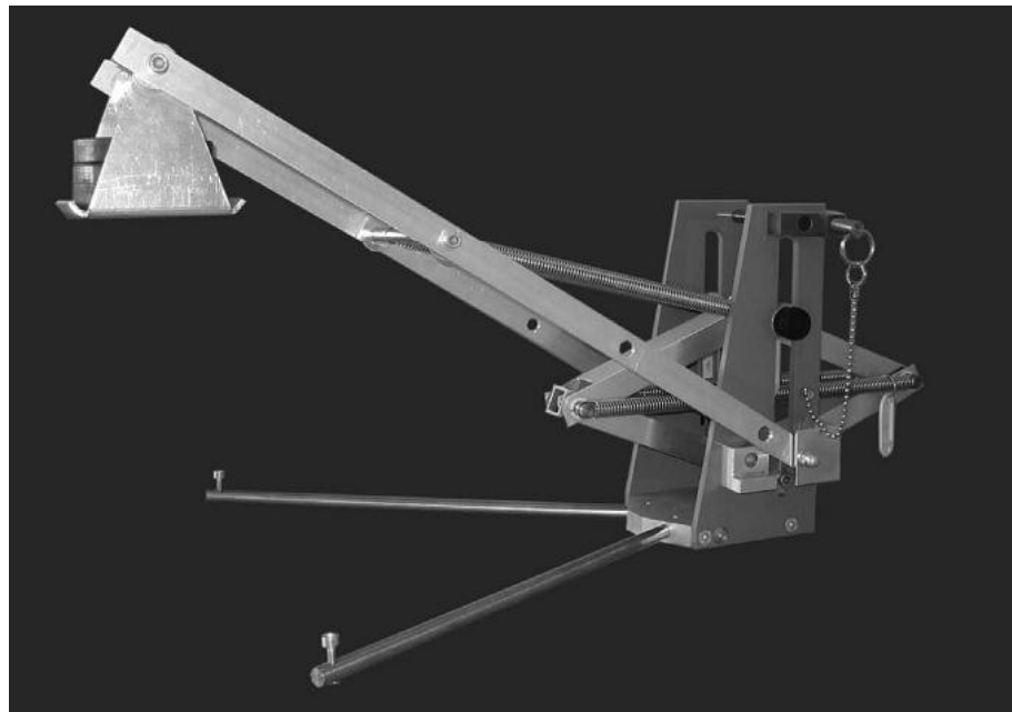
Figure 2.21 – Practical implementation of a gravity equilibrator using the parallelogram storage spring principle with zero-free-length spring ( Barents et al., 2011 ).
