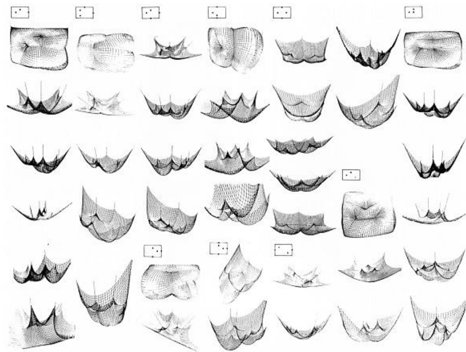
Figure 3.5 – Some possible combinations of suspended nets by Frei Otto.
