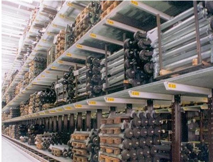
**Figure 1-5. Cantilever racks.**
