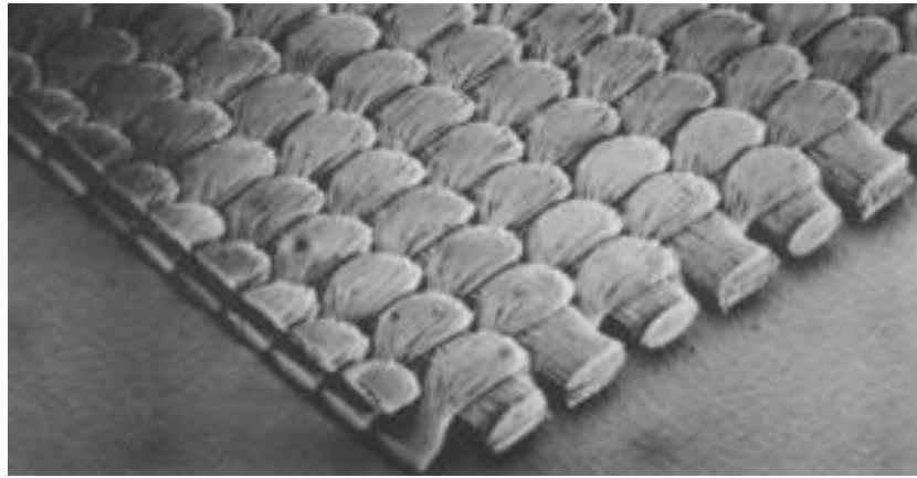
Figure 3.2: The 8.8 oz 1 polyester-Dacron mainsail cloth at 30× magnification. Note low-crimp fill yarns running from lower right to upper left encased by highly crimped warp yarns. This is a fill-oriented cloth.
