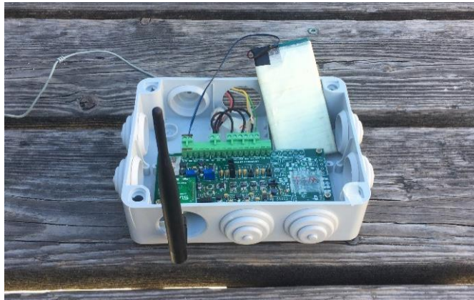
Figure 5.13 WSU employed for the Crossbow data transmission
