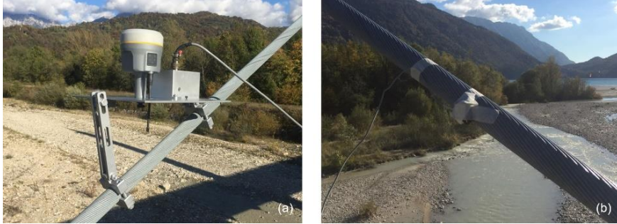
Figure 5.12 147A (a) and Crossbow (b) as located on the footbridge cables
